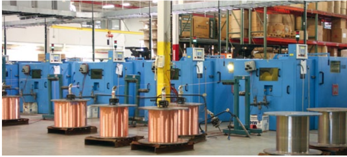
Manufacturing hall with NIEHOFF double-twist bunching machines type D 631
